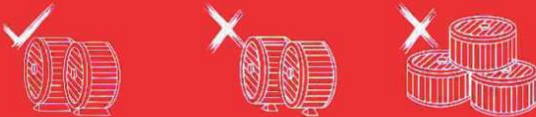
Don't lay drums flat on their sides, use proper stops to prevent drums rolling
