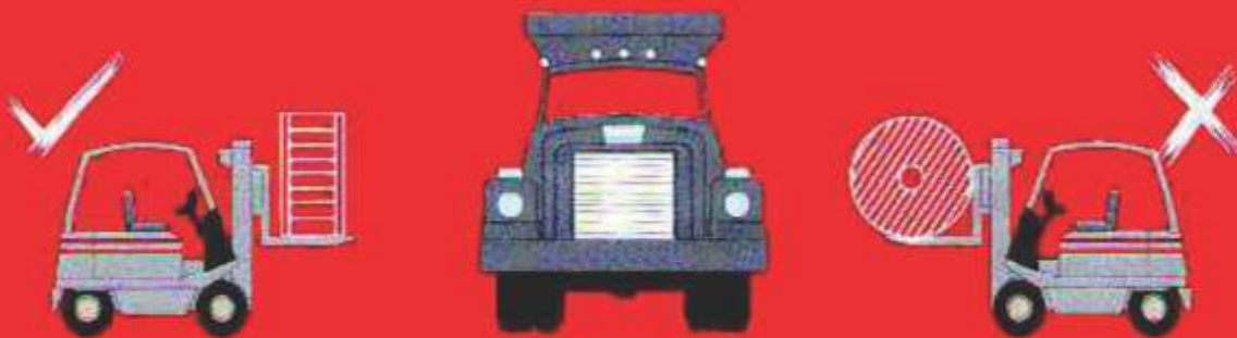
Lift Drums on Fork Trucks
