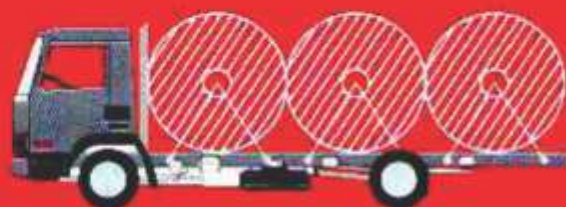
Secure drums adequately before moving
